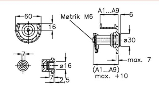
Door + frame thickness = 37-45 Measure type = A5
